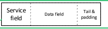
Service field: 16 bit, Data field: MSDU, Tail & padding: Tail: 6 bit, Pad: to fill up last symbol
